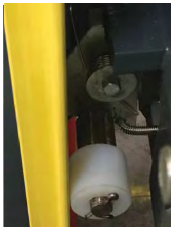
Latch Push Rod attachment.
