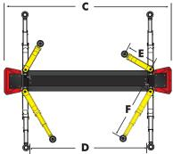
\*Lift capacity ratings are based on loads equally distributed on all four arms.
