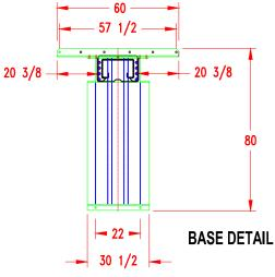
CONCRETE: 3000 PSI, 4" THICK REINFORCED W/ STEEL BAR, MESH
