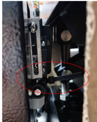
Fig.7.1.3 Wire Ties Position
